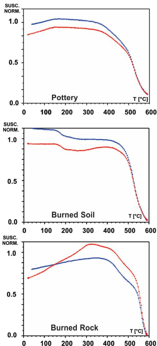
Fig. 2. Susceptibility vs. temperature curves for burned soil, rock and pottery representative samples.
