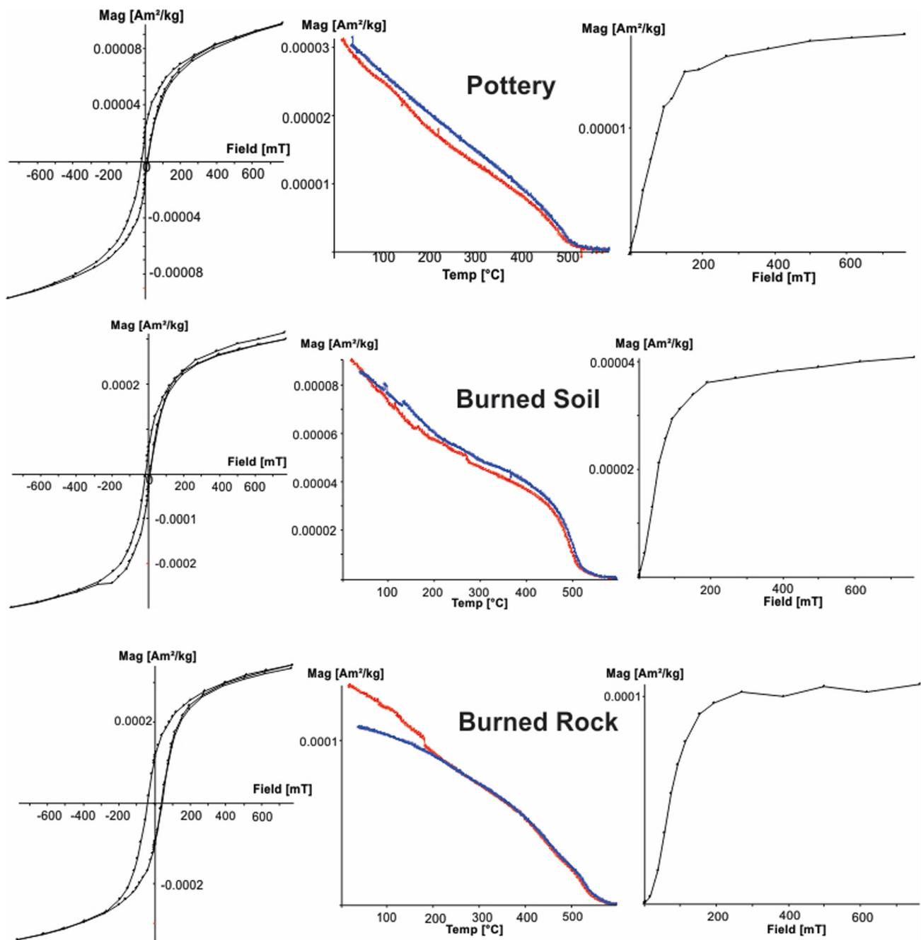
**Fig. 3.** A summary of rock-magnetic experiments for the representative samples: Saturation magnetization vs. temperature curves, the red curve represents the heating curve and the blue to the cooling curve. Hysteresis experiments and associated isothermal remanence acquisition curves obtained with a Variable Field Translation Balance. (For interpretation of the references to colour in this figure legend, the reader is referred to the web version of this article.)
