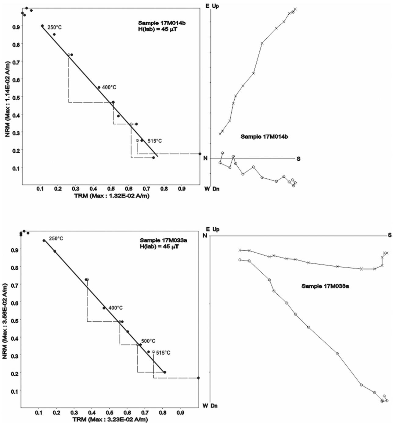
Fig. 4. Representative Natural Remanent Magnetization (NRM)–Thermomagnetic Remanent Magnetization (TRM) plots (so-called Arai-Nagata plots) and associated orthogonal vector demagnetization diagrams for the representative samples.
